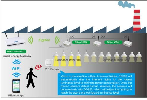
SG200's DI /DO enhance the security management when integrating both motion sensors and security buzzers & alarms
