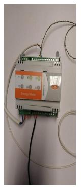
Figure 3b Picture of the 3 phase power meter
