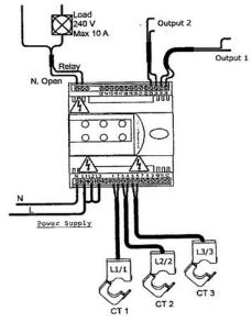
Figure 3a Connection diagram of three phase power meter
